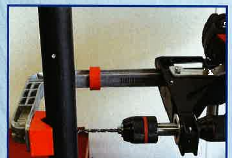
Using Kit #1 with chuck to suit 1mm-13mm twist drills plus holesaws etc.
