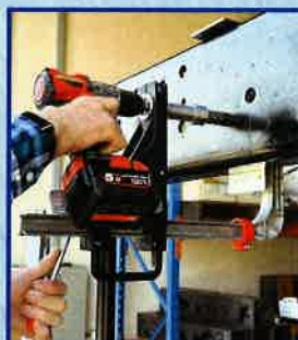
Using Kit #3 arbour with 19mm Waldon Shank broach cutters 25mm DOC
