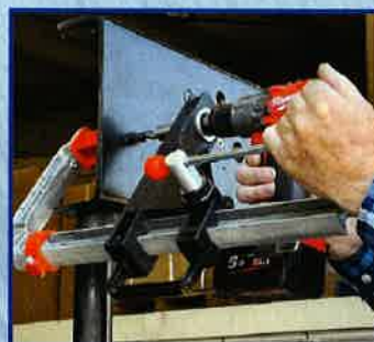
Using Kit #2 with mini cutters from 8mm to 25.5mm Dia. 16mm DOC
